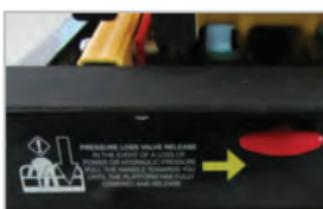
Emergency pressure loss valve release handle
