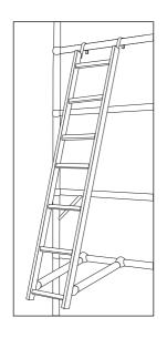
ENSURE THAT CLIP IN LADDER HOOKS ARE POSITIONED INSIDE THE DECK HOOKS, AS SHOWN.
