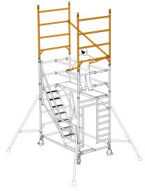
Standing on the fully guardrailed platform, fit the stairway guard rail to the front of the tower. The lower claws fit above and below the cross members of the 2 rung (1.0m) span frame, as shown. Fit the next stair case above the first with the landing claws fitted to the top cross member of the walk through frame.
