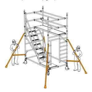
Standing on the fully guardrailed platform, fit a 4 rung (2.0m) span frame at either end of the tower. Fit two diagonal braces in opposing directions, between the 6th and 8th cross members and the 8th and 10th cross members (counting from the span frame end), as shown.
