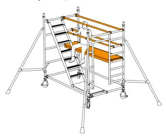
Standing on the fully guardrailed platform, fit a 2 rung (1.0m) span frame to each end of the tower. Fit a diagonal brace between the 4th and 6th rungs (counting at the span frame end) as shown.
