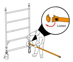
Position the walk through frame as shown and fit the other end of the horizontal brace onto the master rung vertical, just above the bottom casting.
