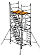
Lock yellow plastic toe board clips over rung and deck claw as shown. Position as (A) on right hand deck claw. On other side of the working platform, position the clip as (B). Place 25mm thick toe boards into slots in toe board clips as shown.
