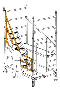
Standing on the stairway, at a height below 1m, reposition the fixed deck to the 5th horizontals (counting at the span frame end). Fit the internal handrail to the stairway. Sitting on the platform, position four horizontal guardrails in line with the edge of the platform on the 6th & 7th cross members, as shown.
