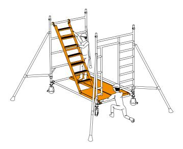
Reposition the temporary deck to the 3rd cross member (counting at the span frame end). Sit on the platform and fit a pair of horizontal guardrails to the 4th and 5th cross members. Climb onto the guardrailed platform.
