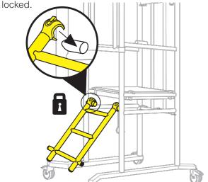
Rotate the ladder down, using the claws as pivots. Locate the bottom of the ladder over the base frame as shown below.
