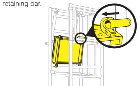
Rotate the platform down and locate the platform claws on the horizontal member of the right hand side frame. Push the platform back towards the back of the unit until it is in contact with the rear folding guardrail frame. Ensure the claws are sitting on the tube and not the plates.
