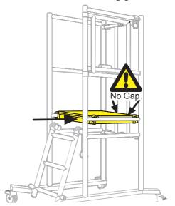
**2** Using the ladder section, climb onto the platform of the work station.
