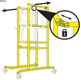
4 Slide the platform towards the front of the unit (the open end) so that the platform claw is clear of the
