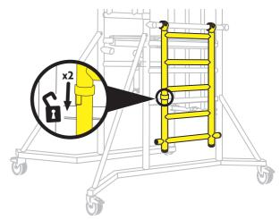
2 Locate the ladder claws over the spigots on the left and right hand side frame. Ensure the claws are
