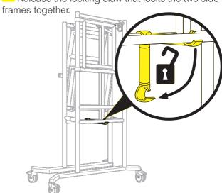
Open the side frames, which will allow the rear folding guardrail frame to unfold. Ensure the rear folding frame is fully open and both elbow joints are locked.
