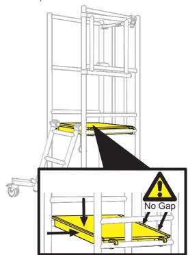
Push the platform towards the back of the unit until it is in contact with the rear folding guardrail frame. Lock the platform retaining plates.
