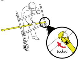
Position the second end frame as shown and fit the other end of the horizontal brace on to the vertical. just above the bottom rung. Fit a second horizontal brace on the bottom rungs on the other side of the frames to square the tower.
