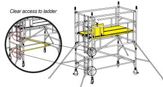
If clear access to the ladder is required, braces may be re-positioned as shown. Reposition braces to original location before moving tower.
