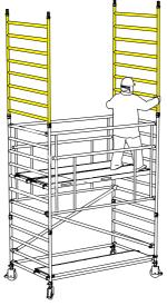
**8** Fit 2 more AGR's to the end frames, with the top claws on the 20th rungs. Fit a trapdoor deck on the 16th rung, with the trapdoor in line with the one below. Place a fixed deck on the 16th rung next to the trapdoor deck.
