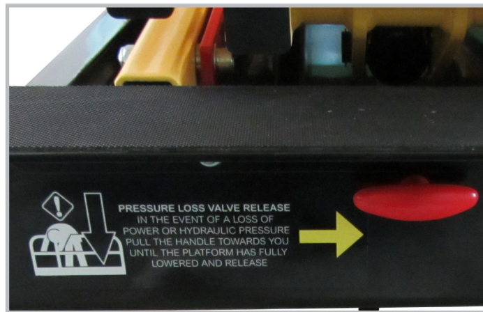
Emergency pressure loss valve release handle
